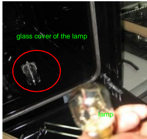
Pull of the electrical connections of oven light
