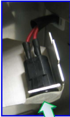
Button Pressed contact closed
