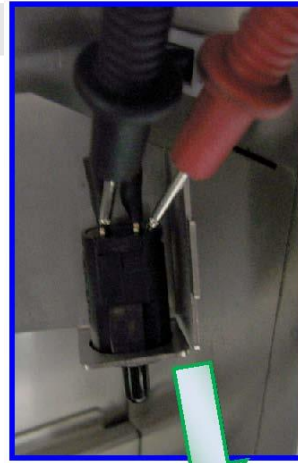
Button Pressed contact released
