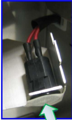
Button Pressed contact closed
